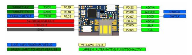
Block Diagram: Connections to use as a programming/debugging interface
